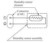
Remark: Do not perform a continuity check of the humidity sensor with a tester. If DC current is applied, it could damage the sensor.
