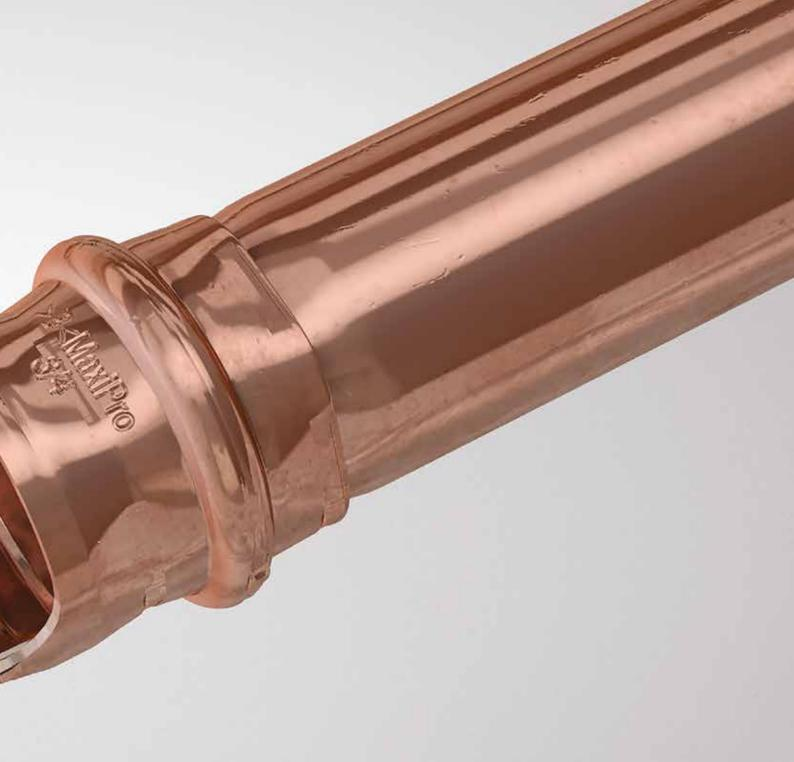
>B< MaxiPro is a press fitting system for use with hard, half hard or annealed copper tube conforming to EN 12735-1, EN 12735-2 or ASTM-B280. >B< MaxiPro provides a secure, permanent leak-proof joint suitable for air conditioning and refrigeration applications.
