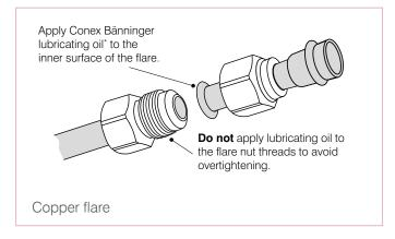
Align the centers of both flares and tighten the flares by hand.
