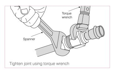
Fully tighten using spanner and torque wrench to the torque values set out in table 9. **Do not over tighten.**
