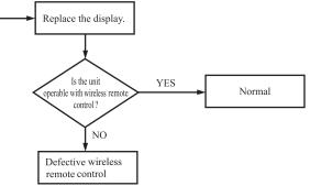
Note (1) Check method of wireless remote control (a) Press the reset switch of the wireless remote control. (b) If all LCD are displayed after one (1) display, it is basically normal.
