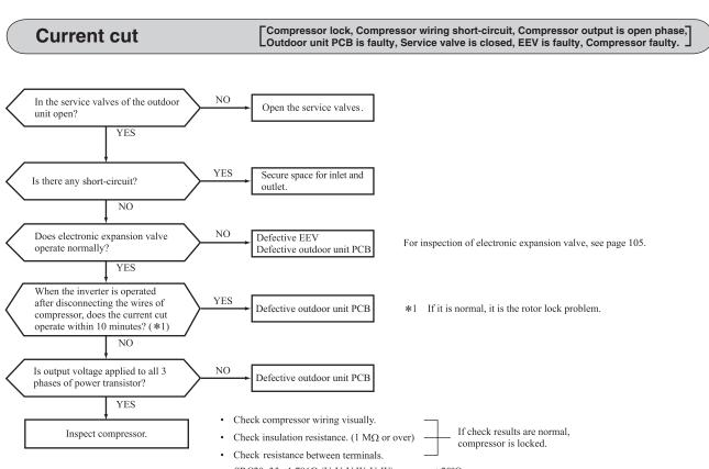
$SRC20-35: 1.786\Omega (U-V, V-W, U-W) \text{ or more at } 20^\circ C$  $SRC50, 60: 1.452\Omega (U-V, V-W, U-W) \text{ or more at } 20^\circ C$
