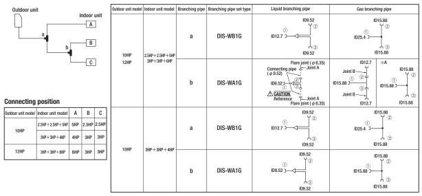
Note When connect the indoor unit of an old model that is shown in the model list, use the joint supplied with the branch piping set like \* A.
