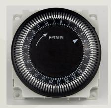
OP-FM1STU00 IS A CAPTIVE-TAPPET 24-HOUR TIME SWITCH MODULE. EACH TAPPET OP-ERATES FOR 15 MINUTES. THE TIMER IS SUITABLE FOR SUB-PANEL MOUNTING. THE 24 HOUR DIAL CONTROLS A VOLT-FREE CHANGEOVER SWITCH, WITH A RESISTIVE RATING OF 16 AMPERES.
