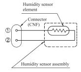
Remark: Do not perform a continuity check of the humidity sensor with a tester. If DC current is applied, it could damage the sensor.
