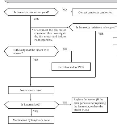
Notes (1) See page 98 for the fan motor and indoor PCB check procedure.
