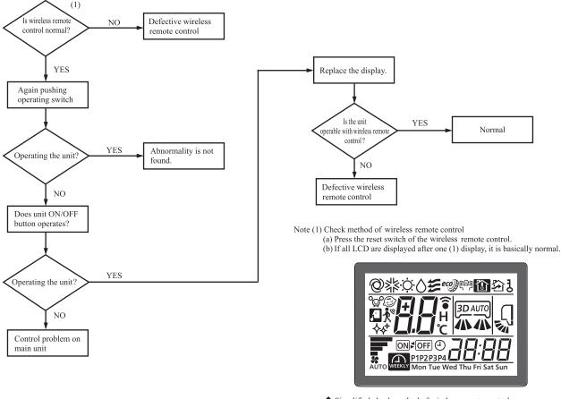
Simplified check method of wireless remote control It is normal if the signal transmission section of the wireless remote control emits a whitish light at each transmission on the monitor of digital camera.
