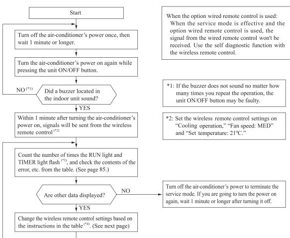
\*3: To count the number of flashes in the service mode, count the number of flashes after the light lights up for 1.5 second initially (start signal). (The time that the light lights up for 1.5 second (start signal) is not counted in the number of
