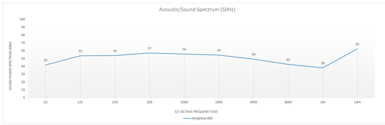
Acoustic spectrum data are calculated by addition of sound power levels of compressor and fan motor at full speed according to EN13215 conditions.
