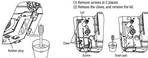
2. Make sure that water drains out completely and that no water leaks from any joints of the drain pipe during the test.
