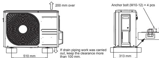
If drain piping work was carried out, keep the clearance more than 100 mm.
