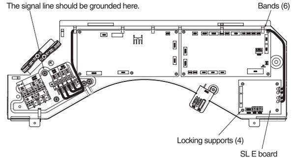
Electrical shock hazard! make sure to turn the power off for servicing. Be cautious so that no abnormal force should be applied to the wiring. Do not let the SL E board hung by the wiring. Do not damage the board with a screwdriver. The board is sensitive to static electricity. Release the static electricity of your body before servicing. (You can do this by touching the control board which is grounded).
