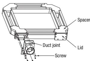
To install the duct joint, screw it in as shown at left.
