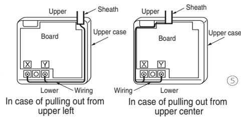
The wiring inside the remote control case should be within 0.3mm<sup>2</sup> (recommended) to 0.5mm<sup>2</sup>.
