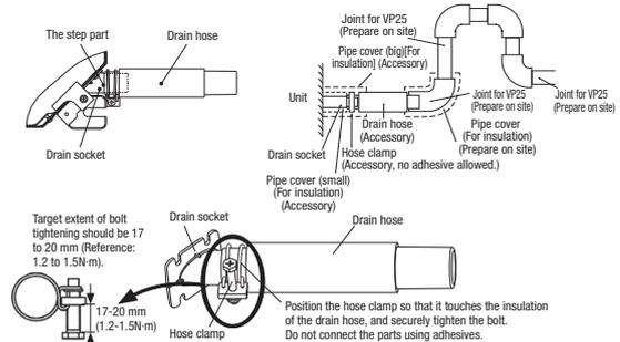
4. Prepare a joint for connecting VP25 pipe, adhere and connect the joint to the drain hose (the rigid PVC side), and adhere and connect VP25 pipe (prepare on site).
