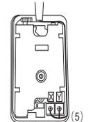
The wiring in the remote control case should be 0.3 mm<sup>2</sup> (recommended) to 0.5 mm<sup>2</sup> at maximum.
