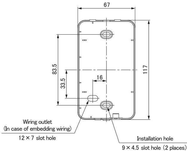
Note: Installation screw for remote control
