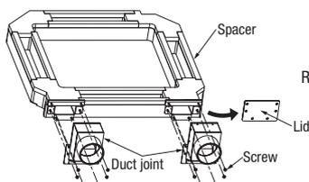
Remove the lid and then install two pieces of duct joint.
