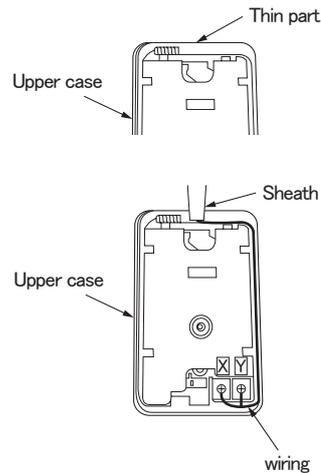
The peeling length of each wiring is as follows:
