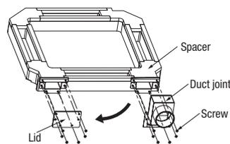
When installing the duct joint at the lid side, remove the lid and reinstall it at the other end before installing the duct joint.
