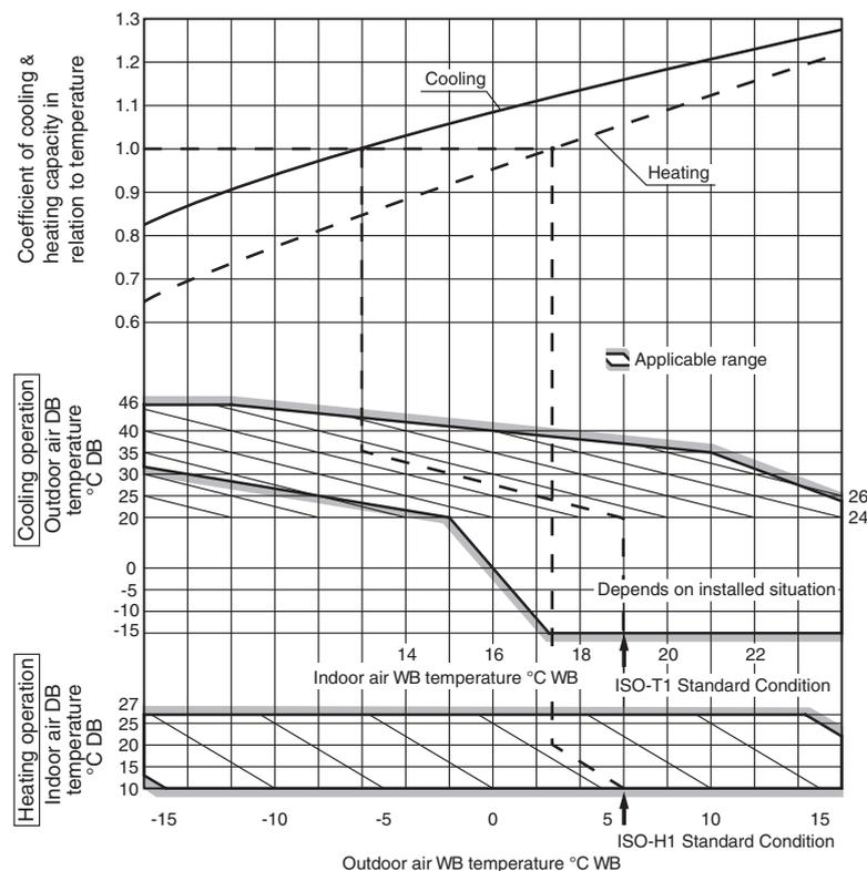
**(2) Correction of cooling and heating capacity in relation to one way length of refrigerant piping**
