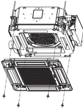
Tighten the panels to the brackets 3 and 4 with bolts.
