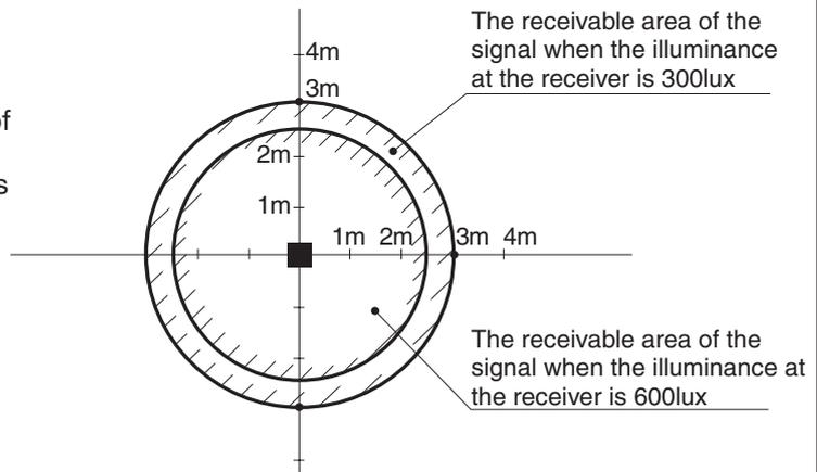
3. Installation tips when several receivers are installed close to one another. Minimum distance between the indoor units which can avoid cross communication is 5m under the condition of 300lux of illuminance at the receiver. (When no lighting is installed within 1m of the receiver in an ordinary office )
