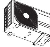
Do not block the drain holes when installing the outdoor unit.
