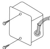
▲ When installed on the back of the remote control, mount it directly on the remote control bottom case.
