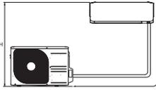
\* Outdoor unit installation position can be higher as well as lower than the indoor unit installation position.
