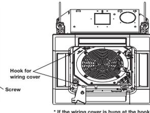
\* If the wiring cover is hung at the hook on panel, it will become easier to work.
