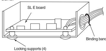
▲ When installed outside the indoor unit, put the metal cover on.
