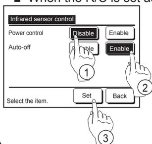
Tap the **Menu** button on the TOP screen and select **Energy-saving setting** ⇒ **Infrared sensor control** or **Motion sensor control**.
