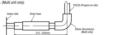
5. Make sure to make descending slope of greater than 1/100 and do not make up-down bend and/or trap in the midway.
