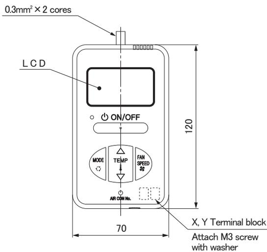
The remote control wiring can be extracted from the upper center. After the thin part in the upper side of the remote control upper case is scraped with a nipper or knife, remove burr with a file.
