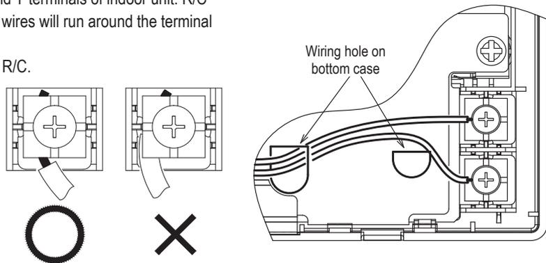
When taking the wiring out from the upper center, open a hole before separating the upper and bottom cases. This will reduce risk of damaging the PCB and facilitate subsequent work.
