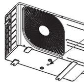
Do not put a grommet on this hole. This is a supplementary drain hole to discharge drain water, when a large amount of it is gathered.
