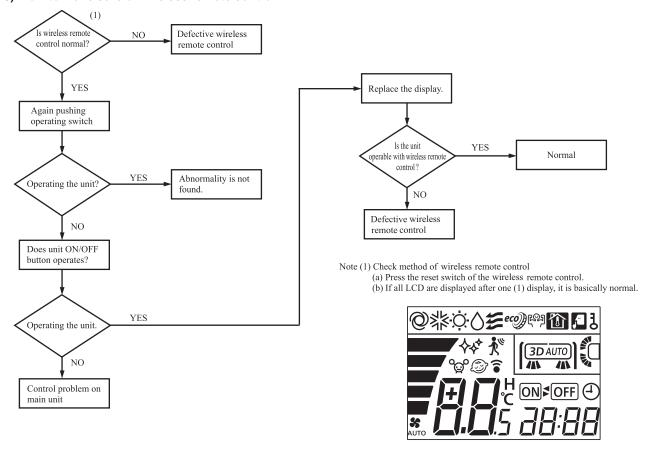
Simplified check method of wireless remote control
