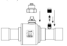
Install valve core with approx. torque 0.3 Nm / 0.2 ft-lbs
